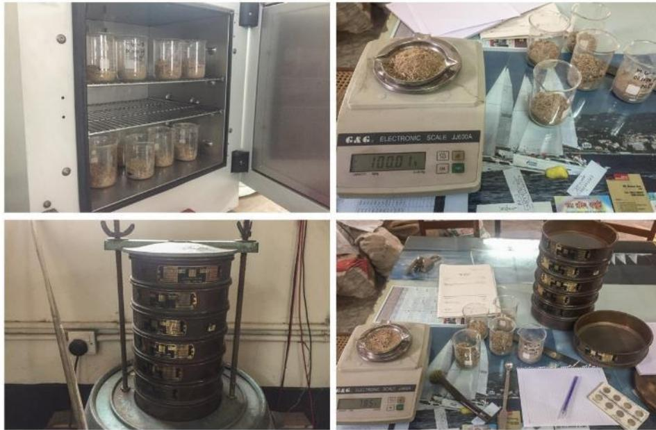
Figure 14: Photograph showing the grain size analysis in laboratory
