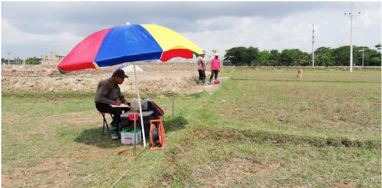
Figure 12: Resistivity Survey [Vertical Electrical Sounding (VES)]
