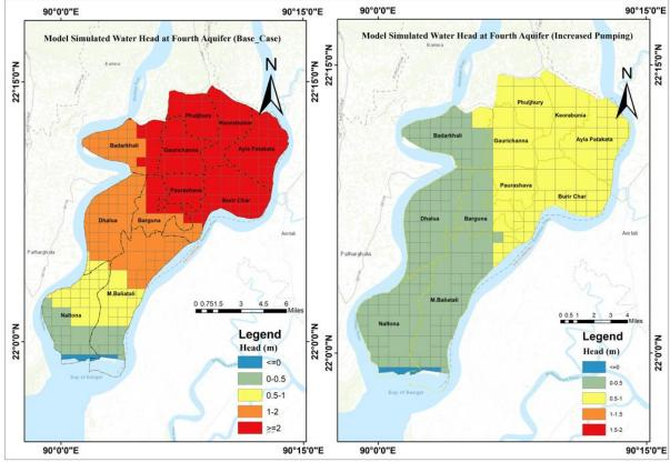
Figure 14: comparison between deep aquifer in Base Case condition in December 2019 (left) and in increased pumping condition in December 2025 (right)
