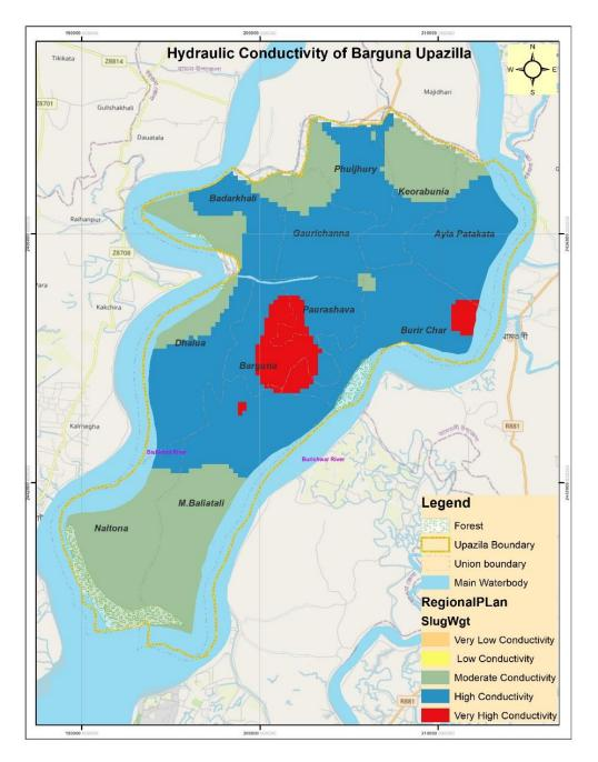
Figure 31: Hydraulic conductivity of Barguna Upazila from Slug test Source: PKCP Project, UDD, 2019
